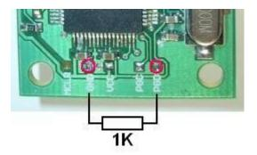
The PGD pad should be pulled down with a resistor (1K) to ground during a Netzer restart.
