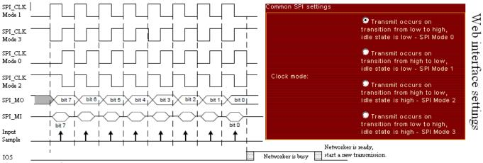
Fig. 2: Waveforms
