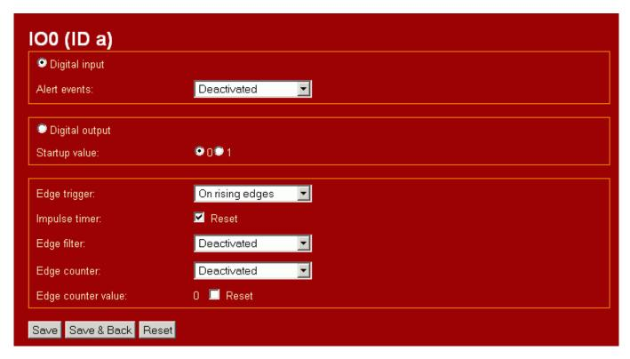
The impulse timer is the core part for generating and measuring impulses on IO3 and SPI\_INT. If the reset check is marked the dedicated impulse timer is reset when the IO0 interrupt occurs.
