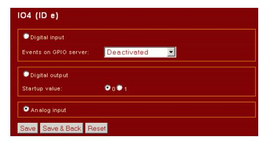
The measuring value is 10 bit (0..1023) in width. It can be queried via the GPIO main page or the  $\underline{\text{GPIO server}}$  or  $\underline{\text{command interface}}$ . The ADC automatically calibrated after Netzer restart. Both channels share the same ADC. The ADC is only activated whenever a readout procedure is activated. The readout procedure takes approx. 2.5  $\mu$ s.
