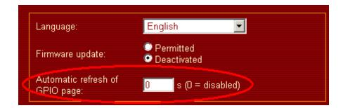
The automatic reload sets after how many seconds the GPIO main page shall be reloaded automatically (in the event of monitoring certain inputs). Reload is activated by the browser, hence the browser is required to support the refresh (look at the browser documentation for this).
