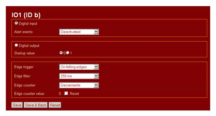
IO0, IO1 and IO2 are provided with edge counters. Depending on the setting, rising or falling edges are counted. The direction of counting (decrementing or incrementing) can be configured. It is a 15 bit counter. Overflows are registered and displayed on the respective IO page. Via the reset checkbox the reading can be reset. The reading and the overflow flag can be accessed also from GPIO server or command interface.
