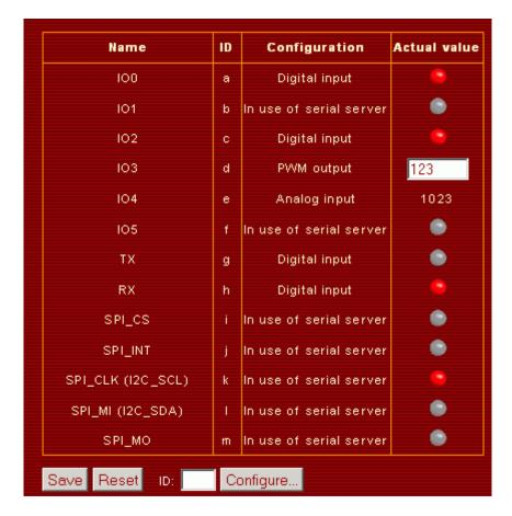
The GPIO main page enables a quick overview and access to all IOs. Digital signals are represented in the form of a checkbox or a ball (depending on whether Javascript is configured. Inputs are exclusively readable. PWM-/pulse values are demonstrated as a text field, hence can be directly changed.
