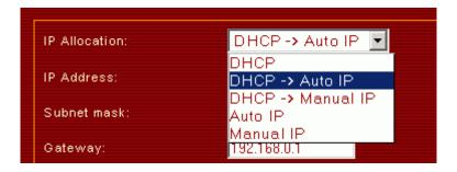
IP mode determines how Netzer allocates its IP address, the subnetwork mask and the gateway.
