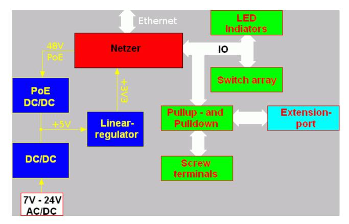
The extension port has an important role. Depending on the application several extension boards can be put in the socket. Extension boards for **LCD** and **domestic** (relays, temperatur and light sensors, opto decoupled inputs) are under development.
