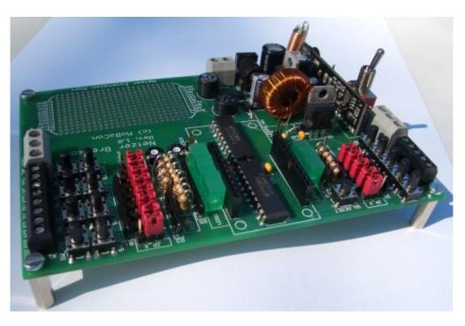
The module has the dimensions 134 mm x 90 mm. All delivered parts are THT parts. The level for assembly is estimated as medium difficult, because of the amount of parts to assemble.
