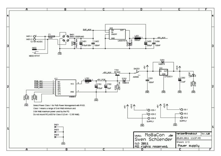
Sheet 2 shows the power supply. The input voltage (6 V – 24 V, AC or DC) from X401 is protected against reverse polarity (B401), ESD (D401) and short circuits (F401). The voltage (SUP\_AUX) is connected to the extension port. The upper part generates from DC or AC with the switching regulator IC4 (in combination with D401, L401 and electrolytes C402 and C403) a stable 5V (+5V\_AUX). A switching regulator was chosen for a wide voltage input range. An extra heat sink is not required.
