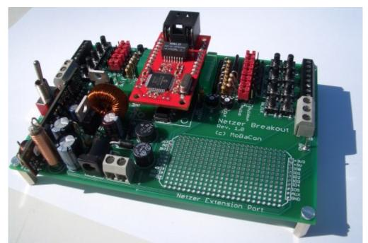
The Netzer Playground enables quick development of circuits around the ethernet gateway Netzer from MoBaCon. Netzer is simply put into the prepared socket.
