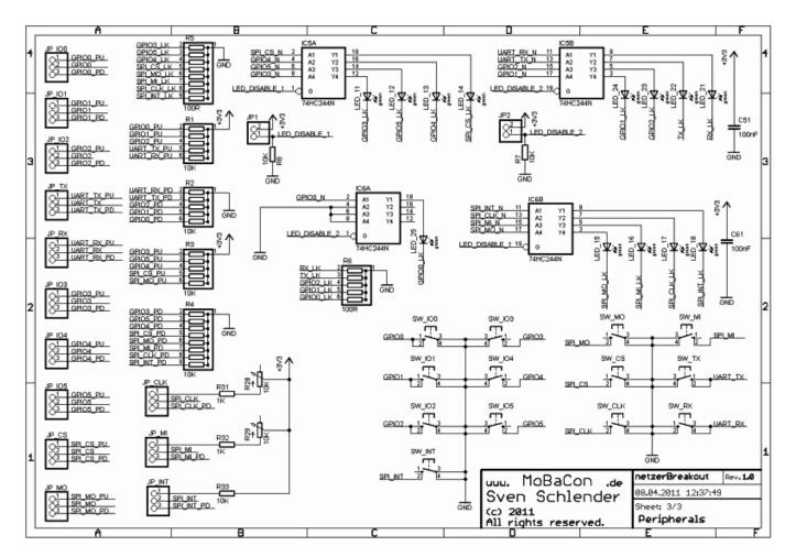
Sheet 3 shows the Breakout parts for testing Netzer IOs. All IOs are connected to LEDs via driver (IC5 and IC6). The LEDs are used as port state indicators. R5 and R6 adjust the LED current. With jumpers JP1 and JP2 the LED drivers can be deactivated as well.
