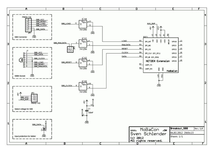
The picture shows a circuit for the Netzer <u>Playground</u> S88 Extension board. The used parts are standard components, which can be build up fast also on a grid-style board.
