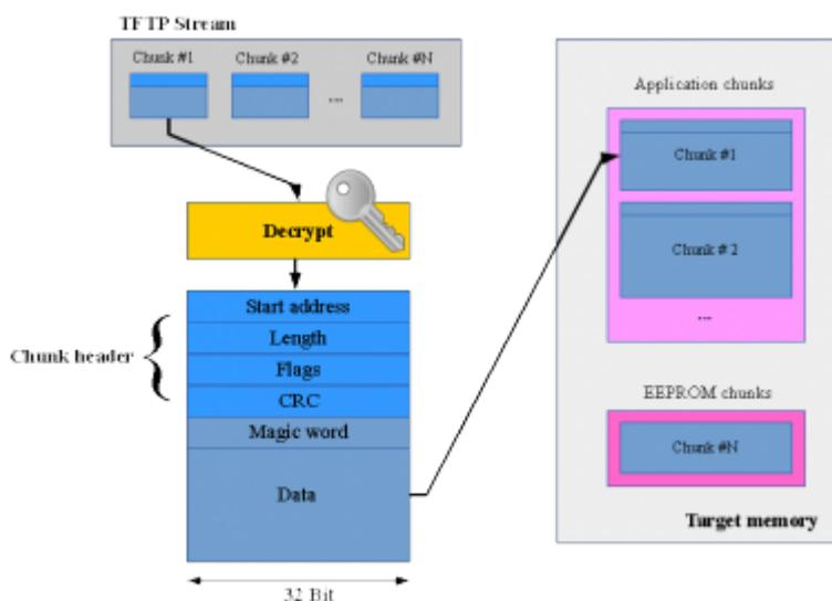
Fig. 3: Uploading chunks mechanism.
