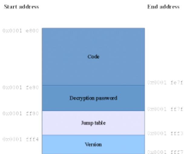
Fig. 2: The detailed structure of the bootloader and its addresses.
