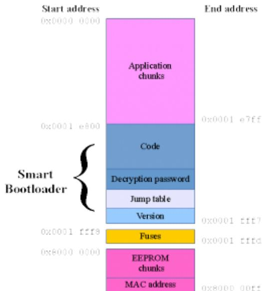
Fig. 1: The whole address region of Netzer with all address positions of the bootloader and the installable application.
